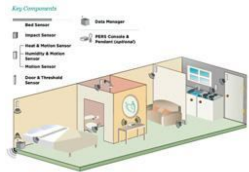
The WellAWARE System is comprised of a variety of sensors in a resident's living quarters. They include impact sensors, humidity and motion sensors, door and threshold sensors and other types of sensors designed to enhance a client's safety and ability to live independently or semi-independently. Opportunity Manor in Sartell is partnering with WellAWARE for a year-long pilot program, which is expected to help fine-tune and bring even more innovations to the system.
